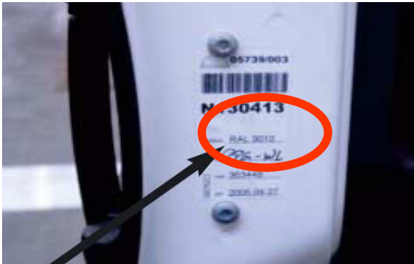
VIN PLATE MAN TRUCKS PAINT CODE LOCATION
